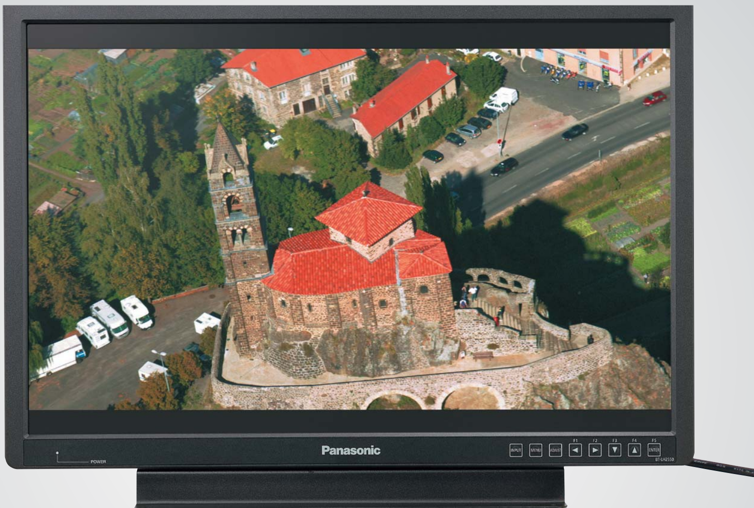
A sample image recorded by an AVC-Intra 100 codec. It is a still image captured from 1920 x 1080-pixel video recorded using 10 bit/4:2:2 sampling.
