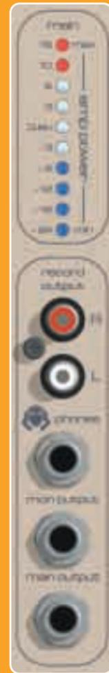
To help achieve optimum volume levels, the GigRac uses a precision, 10-segment, front panel LED meter display, just as you'd find on a professional live sound mixing console. And a further indication that the volume level is too high is provided by an amplifier overload warning LED(s).
