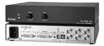
The Extron DVI-RGB 150 converts single link DVI-D signals to analog RGB signals. It is ideal for integrating digital video sources into conventional analog-based A/V systems. The DVI-RGB 150 is equipped with several convenient features for integration such as variable level and peaking controls for the analog RGB output.
