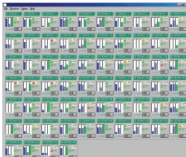
Overall view of all modules. AF-level, antenna signal and the battery status per module/transmitter (name) are displayed. Using the mute switch each receiver can be activated or muted.
