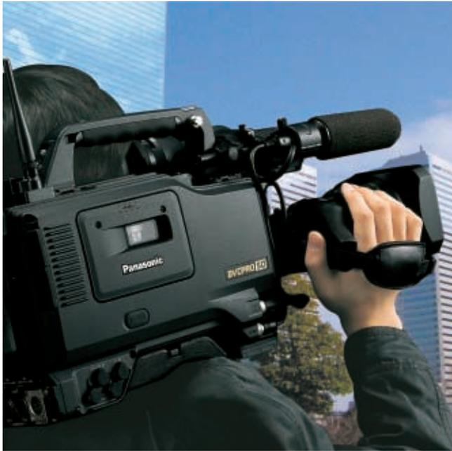
*With the new AJ-SDC905, Panasonic introduces a 2/3" 600,000-pixel 3CCD DVCPRO50 camera-recorder that brings both high quality and high cost-performance to applications from news gathering and sports coverage to content production.*
